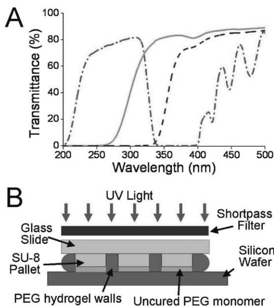
**Fig. 1** Fabrication of a pallet array with PEG walls. (A) UV-visible spectra of a 1 mm thick glass slide (solid line), a 30  $\mu\text{m}$  thick SU-8 film on a glass slide (dashed line), and the 325 nm shortpass filter used for PEG wall fabrication (dash-dot, line). (B) Schematic of the assembly used to fabricate of PEG walls in the inter-pallet spaces.
