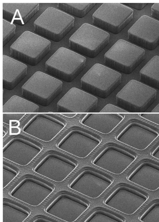
**Fig. 2** SEM images of a micropallet array without (A) and with (B) PEG hydrogel walls. The square pallets possess a side of 70  $\mu\text{m}$  and a height of 30  $\mu\text{m}$ . The spacing between the pallets is 30  $\mu\text{m}$ .
